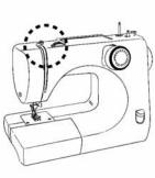
Support the thread on the sewing machine with one hand, using the other hand pass the thread around the thread guide as shown in the diagram.
