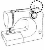
Remove the sticker. Pull up the spool pin from the sewing machine.
